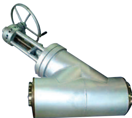
Jacketed Y-valve (300A/250A, Geared operation, 30kgf/cm 2 , 500°C)
