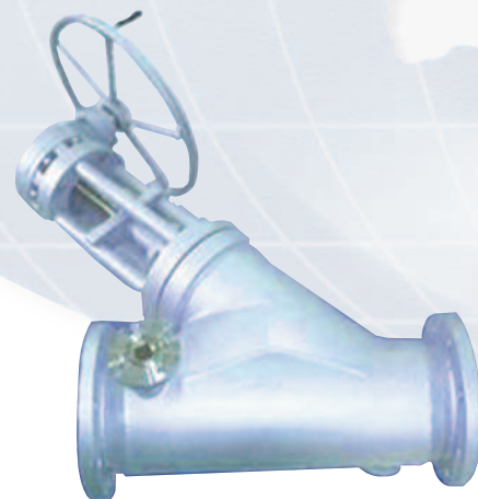
Jacketed Y-valve (200A/150A, Geared operation, 20kgf/cm 2 , 500°C)
